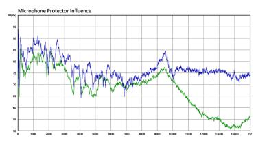
Microphone protector MP21 influences the signal mainly above 10 kHz. Resonances can be attenuated by digital filters
