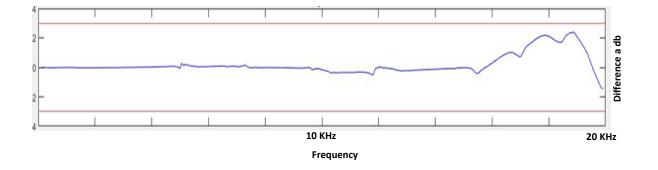
Transfer function for BKS03-D, 3mm compression, 0° angle tilting, stainless steel surface
