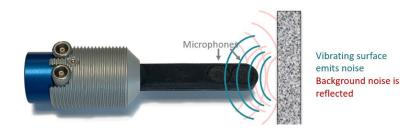
The Discom NFM is designed for a frequency range from 600 Hz to 15 kHz, covering the typical gear mesh and e-motor frequencies relevant for acoustical quality and defect detection.
