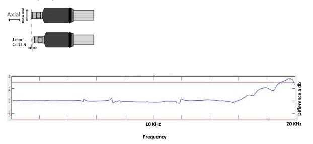
Transfer function for BKS10HD-E, 3mm compression, 0° angle tilting, stainless steel surface
